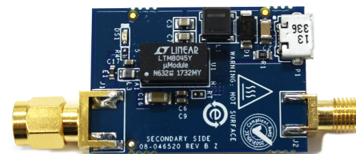
Figure 13. Bottom View of EVAL-CN0417-EBZ Board
